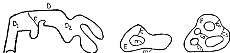
FIG. 12.— D is a simply connected region. E is twofold connected. F is fivefold connected.
