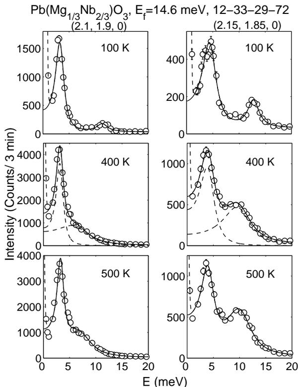
FIG. 4: Constant-Q scans at 100 K, 400 K, and 500 K, are plotted for  $q$  near  $(220)$ . The solid lines are the results of fits to uncoupled harmonic oscillators. The parameters extracted from these fits were used to calculate the structure factors displayed in Fig. 5.
