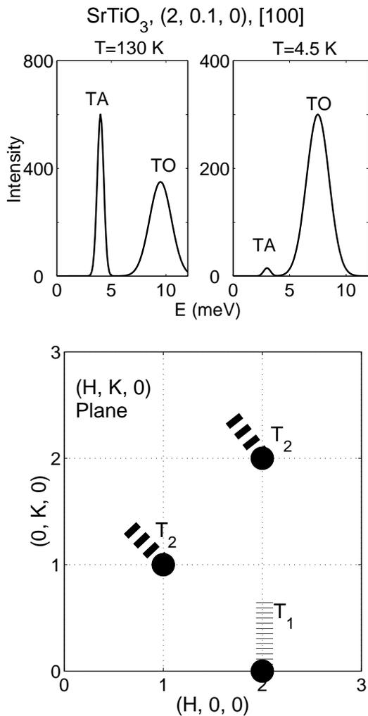
FIG. 1: The upper panel schematically plots the effects of coupling as observed in SrTiO<sub>3</sub> for phonons along the [100] direction as measured in Ref. 15. The lower panel displays the (HK0) scattering plane and illustrates the difference between the T<sub>1</sub> and T<sub>2</sub> phonons. The dashed lines represent the regions in momentum space where the two modes were respectively studied.
