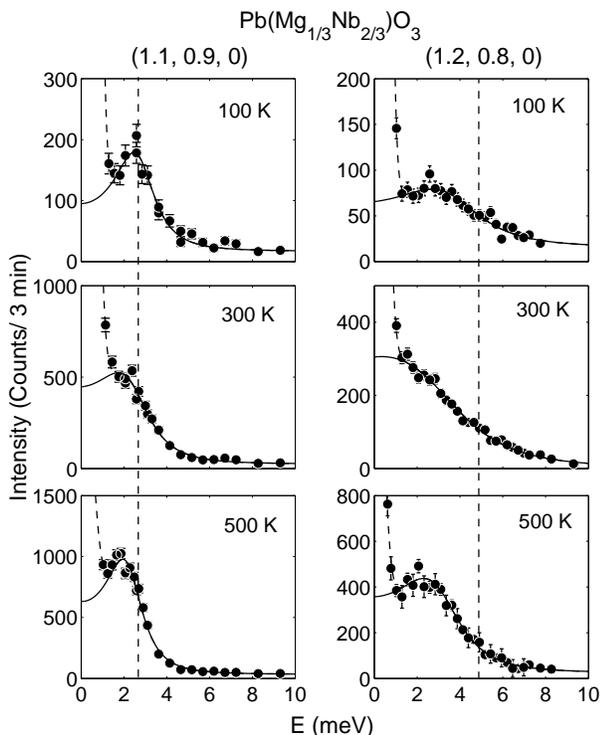
FIG. 7: Constant- $Q$  scans showing the temperature dependence of the  $T_2$  mode near the (110) position. An optic mode was not observable in our measurements indicating a small structure factor. The vertically dashed lines indicate the peak position of the acoustic mode measured in the (220) zone.
